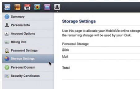
MobileMe uses padded links in its sidebar navigation panel. The large clickable areas allow you to position the mouse cursor over them faster, improving usability.
